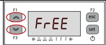
**⚠** The memory of the "clock / date" has a maximum duration of three days, so if the controller is left without power for more than three days, the data set hour / month / year are lost.
