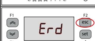
With ERD parameter enable: The water set temperature change on referring the ambient temperature. The function is only active if the temperature precision control is disabled (CPT=OFF).
